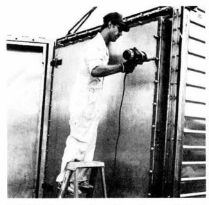
BOLTING the inner door is Dave Bronowski. Each TRUPACT is a steel box within a steel box with eight inches of rigid plastic foam, which serves as shock absorber and thermal barrier, separating the boxes.
